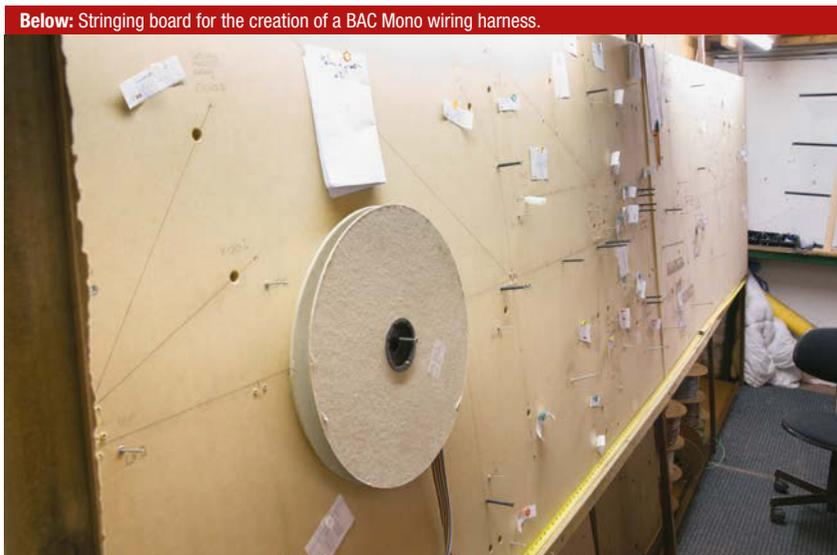
**Below:** Stringing board for the creation of a BAC Mono wiring harness.
