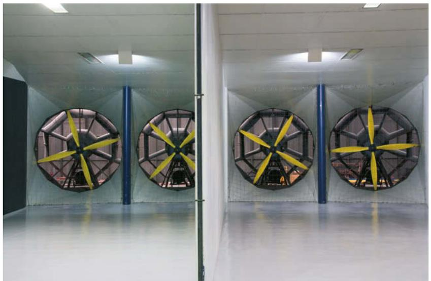
**Above:** Propellers are located behind the test vehicle, pulling air over it rather than pushing from in front.
