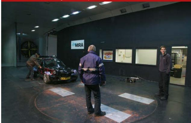
**Below:** Adjusting the measuring plates prior to rolling car into precise position.
